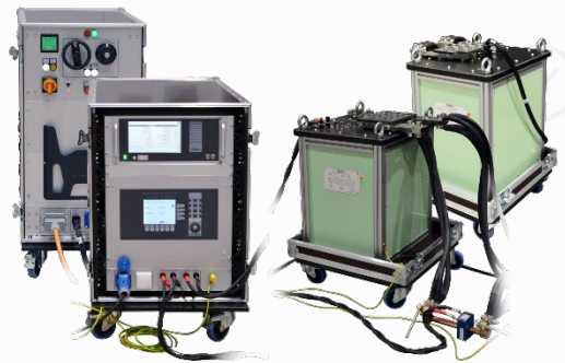
Testing Of Current Transformers
